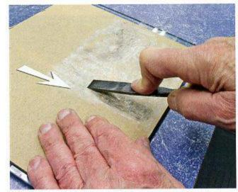
With the beveled surface flat on the rouged cardboard, the chisel is stroked downward while maintaining a constant 22.5° slope.
