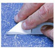
To quickly make a 22.5° angle template (without the aid of a protractor), start by folding the edge of a piece of paper to produce a 45° angle.
