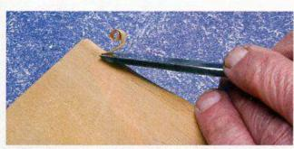
Test the chisel's sharpness by cutting on the edge of a piece of wood. If it shaves a curl of wood as shown, your chisel is ready to carve cleanly. If not, repeat a few of the sanding steps, beginning with 600-grit paper and gradually incorporate finer sheets.
