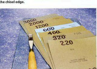
The next several steps consist of using progressively finer silicon-carbide paper, moving from 220-3,000 grit. On each successive sheet, follow the procedure in the previous two steps. First, stroke the flat side, then the beveled side. Smaller burrs will continue to form, and the beveled surface will become smooth and reflective.
