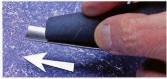
The other difference with gouges is the step involving the flat, non-beveled side's burr removal. The flat stroke is easily accomplished by rolling a small piece of 600-grit siliconcarbide paper and stroking the gouge as shown.
