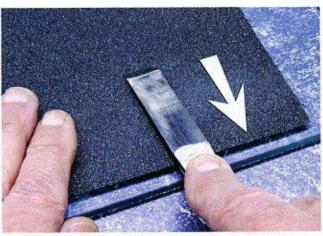
The flat (non-bevel) side of the chisel is stroked with downward pressure 15-20 times. Eventually, a burr will form at the chisel edge.
