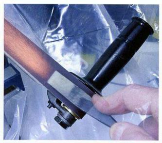
To shape the chisel at the correct bevel angle, hold it at the 22.5° angle over a belt sander running with a 60-grit belt. The belt should be moving away from you. Maintaining the constant slope is important. Once it's done, this step doesn't need to be repeated; it simply creates the required 22.5° bevel slope.
