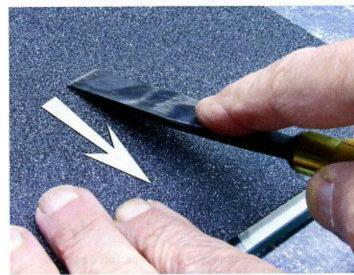
Next, the beveled side is stroked downward at a constant angle of 22.5° for 15-20 strokes. The burr that formed in the previous step will be eliminated, and a new burr will form on the beveled edge.
