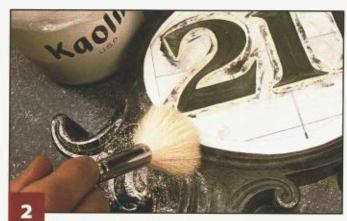
Dust the surface with kaolin USP. Vacuum up the sanding dust, wipe it with a paper towel, and vacuum again. Spatter the kaolin, a pure powder form of the mineral kaolite, on the entire surface of the sign and smooth it out with an artist mop brush. Vacuum away any excess dust. The kaolin make the colorless size visible and also prevents gold leaf from adhering to the painted areas on the cove and scroll that are not intended to be gilded.
