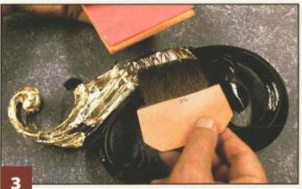
Apply the gold leaf. Transfer the gold leaf to the sized surface using the gilder's tip lightly charged with lip balm. The gold leaf is attracted to the oil on the brush, but is more attracted to the size and will easily transfer to the size.
