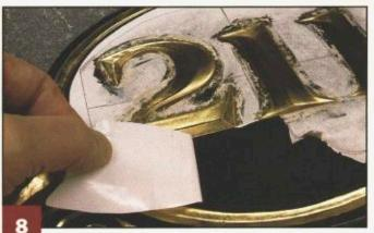
Remove the vinyl mask. Use a hobby knife to lift up a corner of the mask. Pull the vinyl at a 90° angle to the gold-leafed edge. Cut the mask with scissors at strategic places, such as the serifs, to facilitate crisp clean edges. If you pull the mask toward the gilded section, it may lift some of the gold. Always remove the vinyl mask perpendicular to the gilded edge, not toward it.
