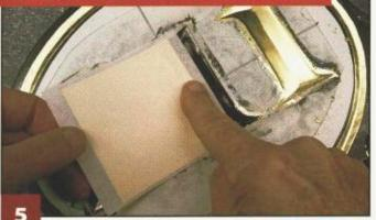
Gild the cove and numbers. Let the size dry for two days. Start at the top of the cove and work your way around. Place a sheet of gold leaf face down on the size and press lightly. The gold should rest on top of the size, but not be submerged in it. The gold peels off the paper as it sticks to the size. Gild the numbers, pressing lightly on one side of the number and then the other.
