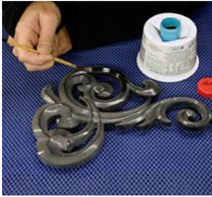
Using Smooth-On's dye, he coated the cast pieces before gilding.
