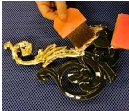
After a kaolin dusting and smooth-size application, 23½k surface gold adds brilliant sheen.
