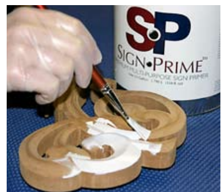
Before the casting process, he coated them with Sign Arts Products' Sign*Prime™ all-purpose primer.
