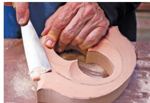
Gouges are used to carve the prismatic profile. Tight curves require greater sweeps. A lesser-sweep gouge, such as No. 2, can be used to carve the outer surfaces.
