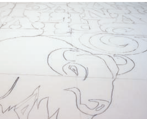
Letters, outlines and the logo are transferred to the HDU, ready to be cut out.
