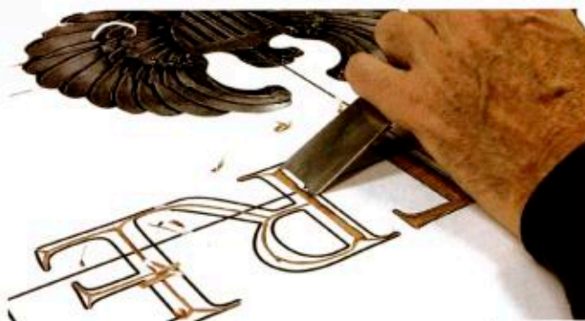
Using a No. 2 sweep gouge, Francis made rough cuts into the letters' surface. To refine his dimensional carving, he used a #1 sweep straight chisel.
