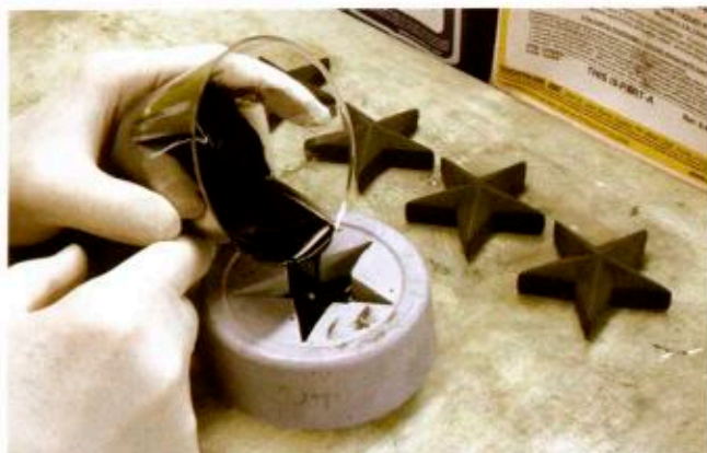
Using Smooth-On's moldmaking and casting compounds, Francis created molded stars for the signface. This molding system allows him to replicate designs.
