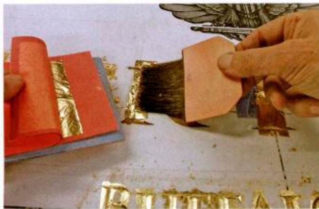
Using a gilder's tip, Francis applied the cut sheets to the surface.
