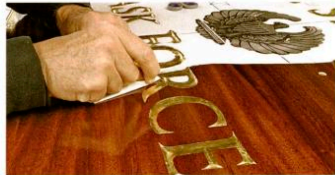
After having gilded the letters, Francis carefully removed the vinyl mask. He strongly advises against pulling the film towards the letters' edges – rather, he said the fabricator should pull the media away at an upright, 90° angle.
