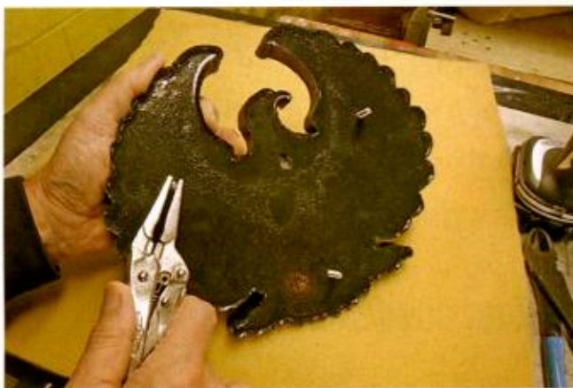
Francis inserted three, threaded, aluminum studs to the eagle applique's underside.
