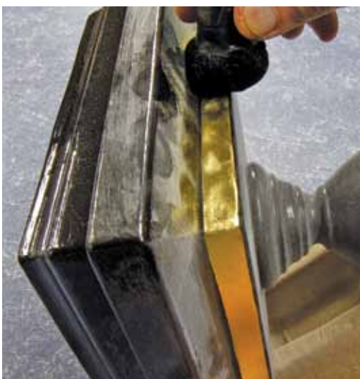
To help the cap's flat surface reflect light more attractively, we etch the goldleaf by engine turning with velvet-covered cotton.
