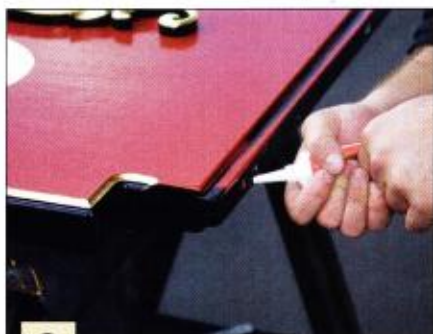
8 Pilot holes for the lag screws were previously drilled and are filled with 100% silicone.
