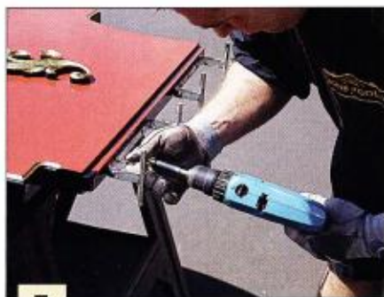
5 We remove the handles from the panel's edge.
