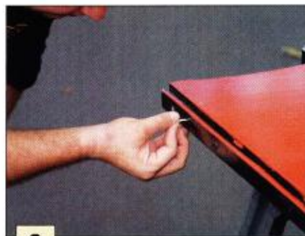
6 Fill the screw holes with wood epoxy.
