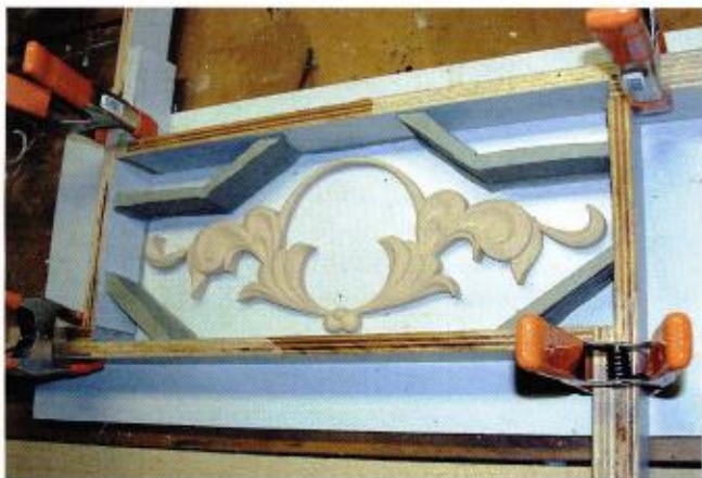
Francis constructed MDO board to form a confinement field, and then created interior walls with modeling clay. Creating clay barriers conserved the amount of molding material by up to 25%.
