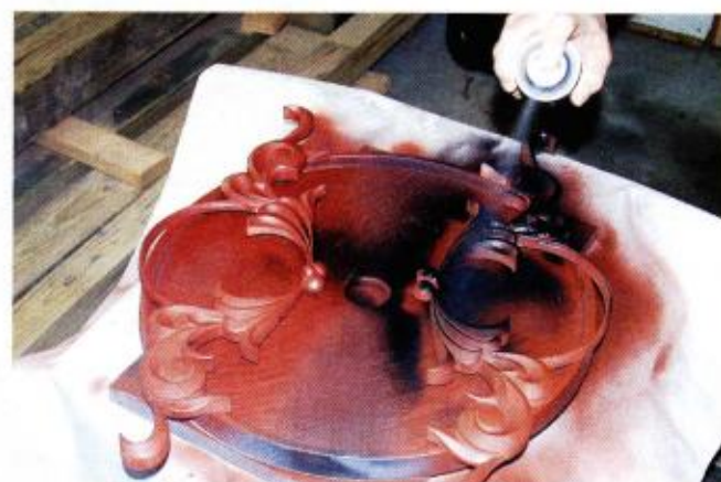
Francis began decorating the casting by applying Krylon™ automotive primer, then allowed 30 minutes to dry. Next, he used several coats of black Krylon spraypaint.
