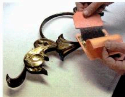
After applying slow size to the casting and letting it cure for 48 hours, Francis used a gilder's tip to apply looseleaf, 23k, double gold.
