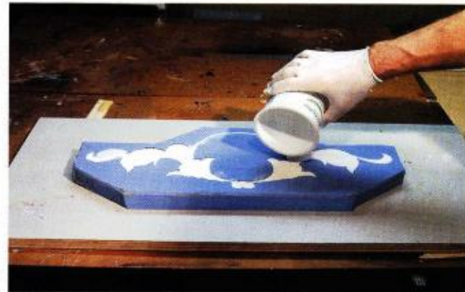
Francis poured in the casting material. Like the mold material, it contains two components. It's vital that the mold is free of moisture before casting; otherwise, the casting mixture causes a heat-emitting reaction that vaporizes water, leaving hollow spots.
