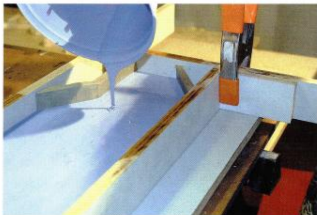
He poured equal amounts of the two-part molding compound, Smooth-On's OOM00-30, into the field; one part serves as the molding base, while the other functions as the curing agent.
