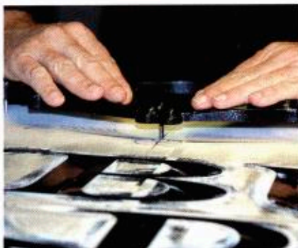
To determine the casting's location on the sign, he used a template that he positioned amidst the sign's other elements. By pressing on the scroll firmly, the studs slightly imprint the mahogany's surface, leaving drilling marks.
