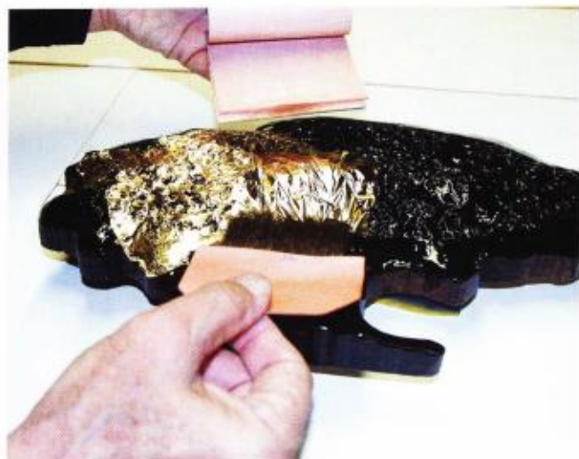
Using a gilder's tip, Lestingi applied 23k looseleaf, double gold.
