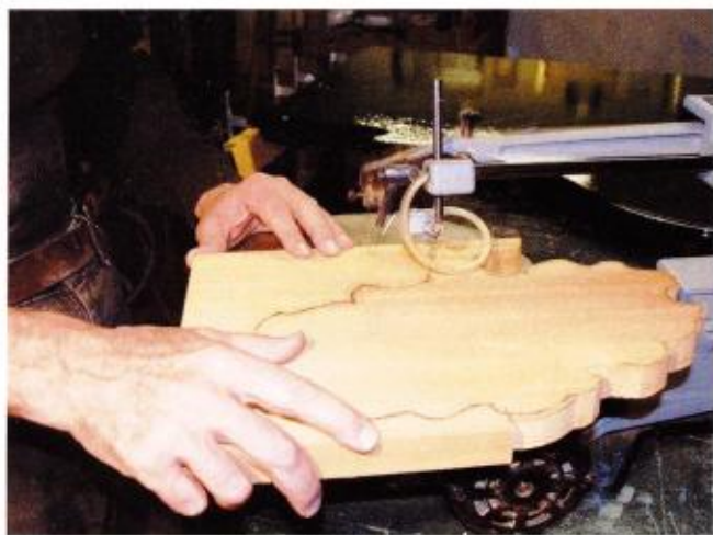
Using a scroll saw with a spiral blade, Lestingi cut out the tree. A saber saw would work, but a spiral blade can move a substrate in any direction while cutting — a time-saving step.
