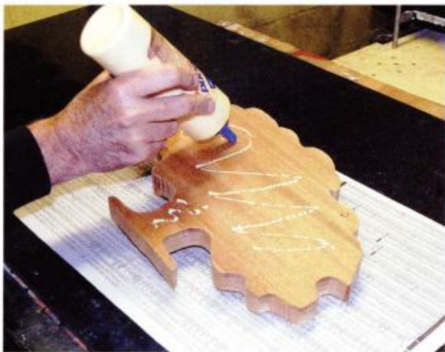
Lestingi applied a zig-zag pattern of yellow carpenter's glue, which provides strong adhesion with only a moderate application.
