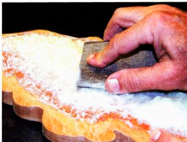
After the epoxy hardened, he used 60-grit sandpaper to initially sand the surface, and finished with 120-grit sandpaper.
